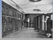
While programmable for different tasks, ENIAC's programs were a series of switches and wires plugged into specific orders.
