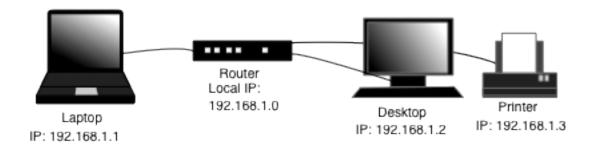
The client/server model of network traffic continues as above. However, instead of the laptop making requests to the desktop, the request will go directly to the printer that is connected to the router.
