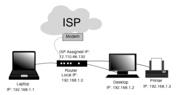
In the example illustration above, the router gets its own IP address from the ISP then translates IP addresses for traffic between the local network devices and the wider ISP network and internet.
